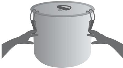
The closure of the lid has to be carried out in closing 2 hooks on the opposite sides simultaneously, in order to obtain a homogeneous pulling of the lid and thus avoiding dislocations and subsequent coupling defects of the springs.
